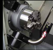
Pre setting arm in the tool measurement position
