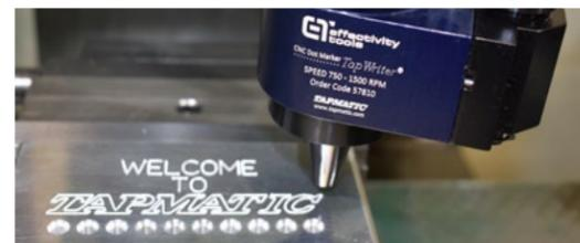
Mark logos using standard CAD/CAM software for the tool path.
