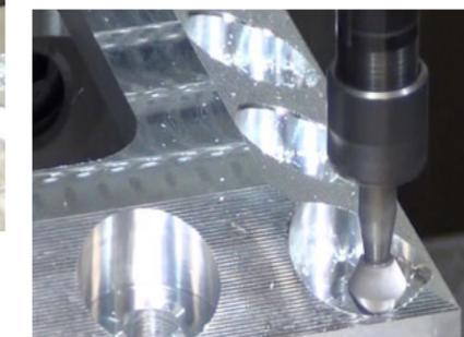
**Chamfering holes on a curved surface presents a problem for conventional methods.**
