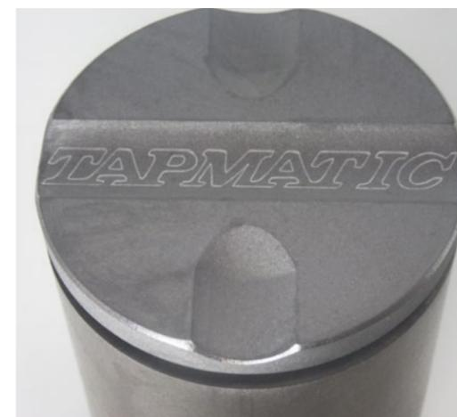
**The DeBurr-Z can also be used for engraving. It allows a faster approach to the work piece and the ability to mark on curved surfaces. We offer combination deburring/engraving cutting tools.**
