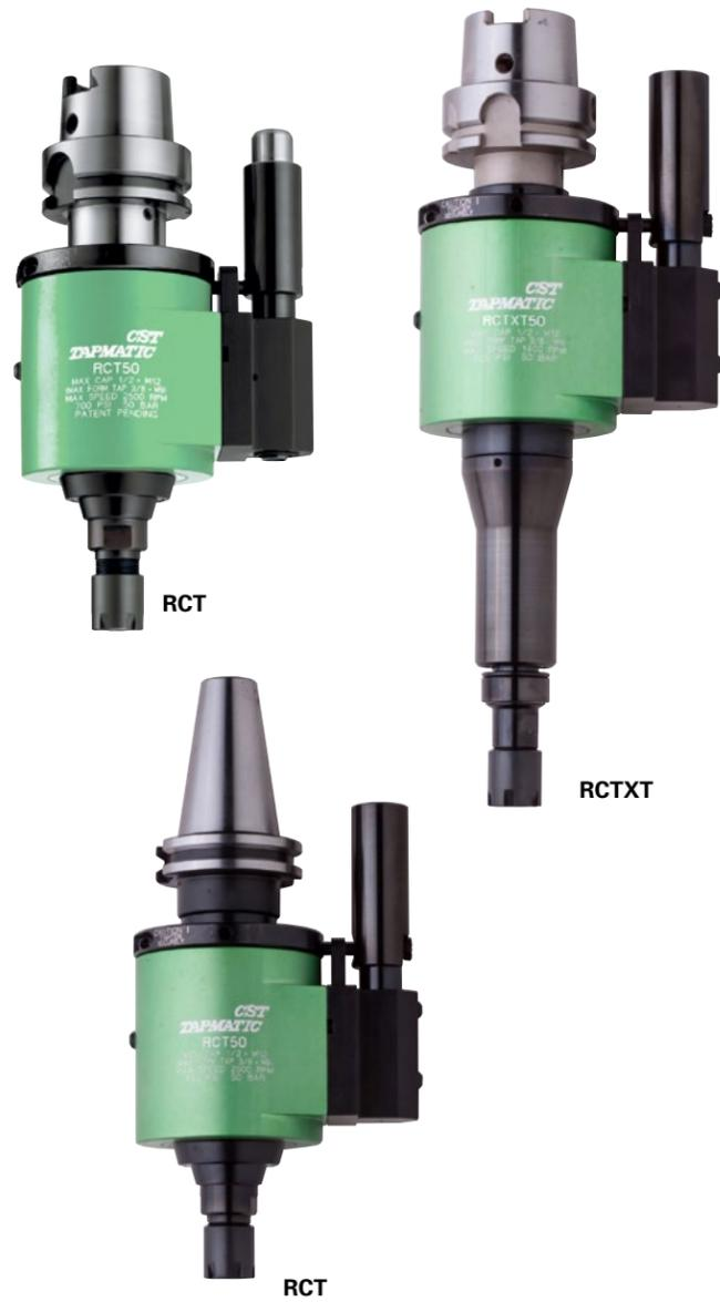
CST Constant Speed Tapping relies on a compact tapping attachment to provide tap reversal. The machine spindle runs in one direction at the exact programmed speed and reversal occurs within the tapping attachment instantaneously upon machine retraction. This avoids the inevitable RPM fluctuations which occur with reversal of the machine spindle. Benefits include the following...
