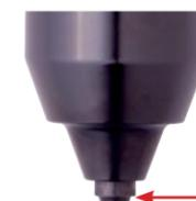
Simply unscrew the stylus holder to remove it.
