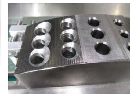
**Going around the holes with the axially floating DeBurr-Z produces consistent results.**
