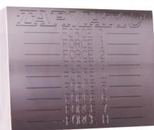
Example in 4140 pre heat treated material with hardness 28 HRC. Marking at different settings with 1.3 mm compression against the surface.
