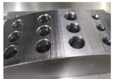
The DeBurr-Z can also be used for engraving. It allows a faster approach to the work piece and the ability to mark on curved surfaces. We offer combination deburring/engraving cutting tools.
