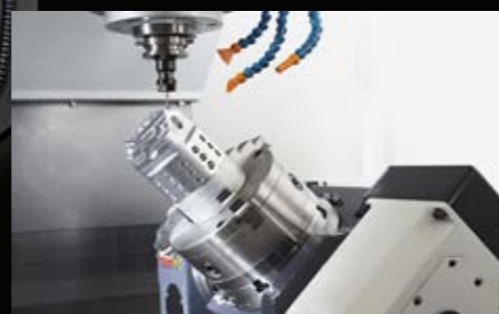
5th axis option is available on all XYZ Vertical Machining Centres except the LR Range.
