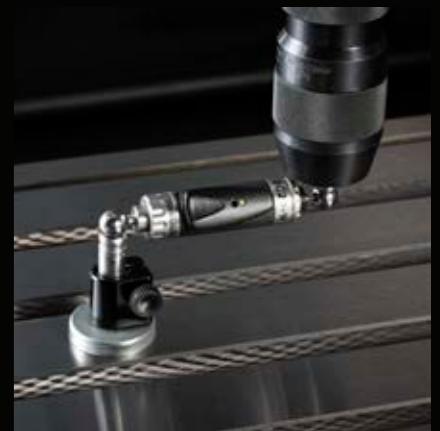
All ProtoTRAK Turret Mills and Bed Mills are Renishaw ball bar tested to ensure accuracy.
